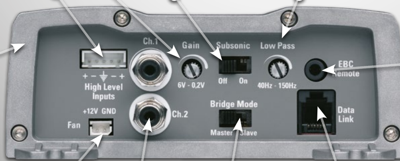
Thermo regulated connector for external cooling fan(s)
