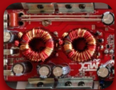
Dual power transformer (To improve the cooling and the reliability)
